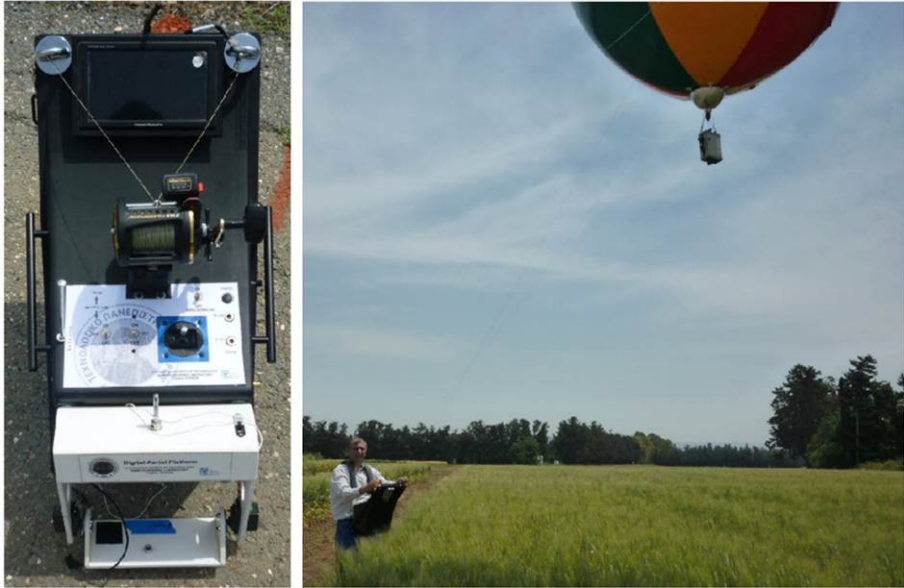
Figure 27. Right- ground control mechanism and aerial platform. Left-Low altitude airborne system including air balloon, spectro-radiometer, and researcher wearing ground control mechanism with harness (Themistocleous et al., 2012b)
