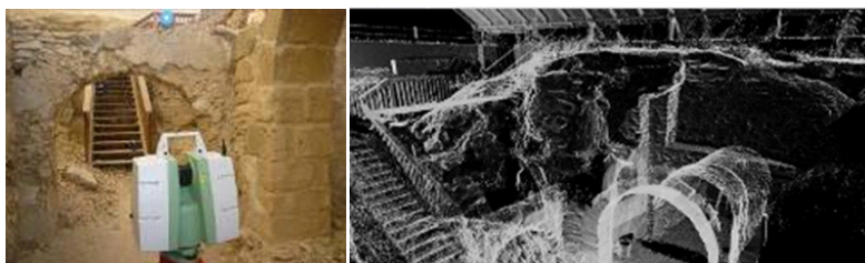
Figure 19. Data collection from the church of Saint Theodore in Idalion village (left). Registration of the point clouds for Saint Theodore in Idalion village. All point clouds are transformed into one coordinate system (right) (Agapiou et al., 2010b).
