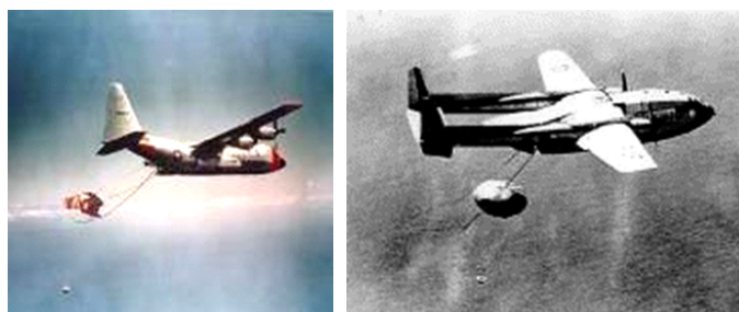
Figure 1. Film capsule of the CORONA satellite collected from aircrafts. (Photos from Wikipedia and CSNR collection)
