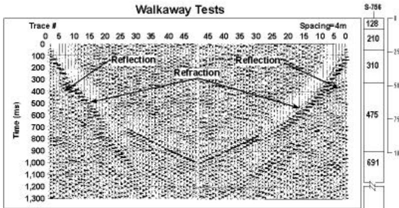
Figure 3. A reversed SH-wave walkaway test of average quality from northeastern Arkansas. The interpreted depth-velocity model (in m/s) for the site is shown at the right. The shear wave velocity of the deeper sediment (below approximately 100m) was not sampled. The 846m depth to bedrock (shaded) was determined by P-wave soundings.
