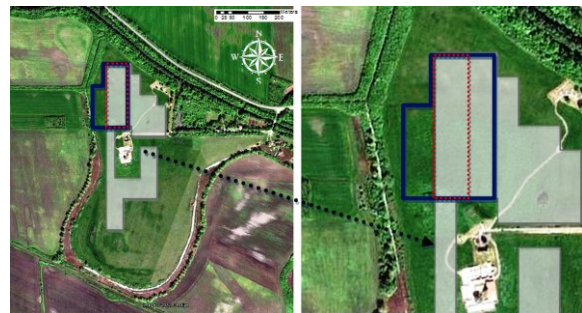
Figure 2 Left: Entire area of the Vészto-Mágor Tell covered from the different remote sensing techniques; Grey and blue polygons indicate the area covered from the geophysical surveys (GPR and magnetic respectively) while red polygon indicates the area covered from ground spectroradiometer. The whole area of the Tell was also captured from satellite images (not indicated with polygon). Right: Detail map from the common area covered from all remote sensing techniques (geophysical; satellite image; ground spectroradiometric measurements) (background Google Earth) (Sarris et al. 2012).
