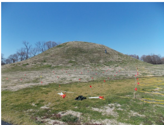
Figure 1 View of Mound B at Toltec Archaeological Park from the south. The flags denote the position of the electrodes used to collect the ERT data.
