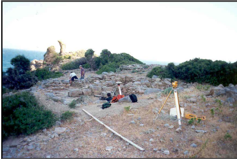
Figure 4 : Simultaneous mapping with GPS and EDM at Chalinomouri, E.Crete
